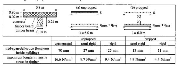
Table 1 Example of deflection and stress in a timber-concrete composite beam. The construction process (propped/unpropped) and the rigidity of the connectors are important parameters
