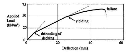
Fig. 4 Pre-Fire Load/Deflection Results for Internal Panel
