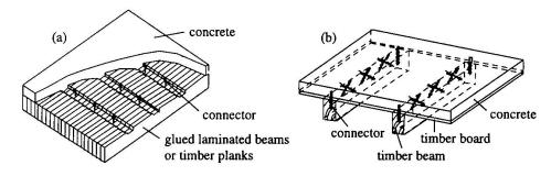
Fig. 2 Design of timber-concrete composite floors: slab type floor (a) made of glued laminated beams with the longer side of their cross-section horizontal or nailed laminated wood of sawn timber planks and beam type floor (b) with glued laminated or sawn sections
