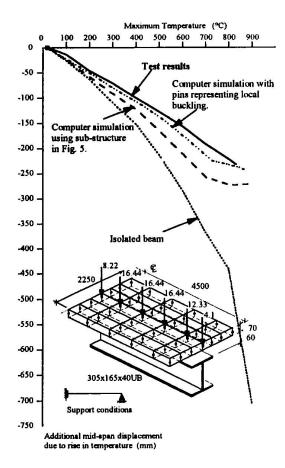
Fig. 2 Comparison between computer predictions and test results.
