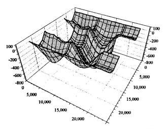
Fig.6. Deflection of large compartment at 730°C.
