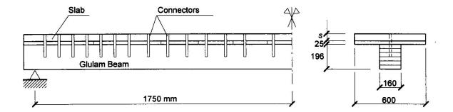
Fig. 1 - Full size samples of the tested timber-based composite structure.
