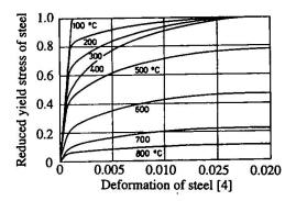
Fig. 6 Reduced strength and stiffness for timber and hot rolled steel at elevated temperatures
