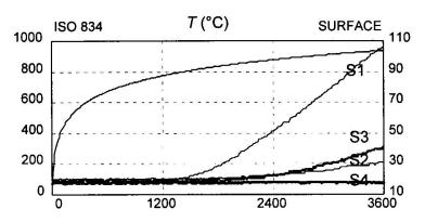
Fig. 2 - Maximum temperatures at the unexposed floor surfaces.
