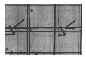
Fig. 5 SFS connector. It consists of a self-drilling screw with a collar to limit the screwing depth and a head for connection with the concrete.
