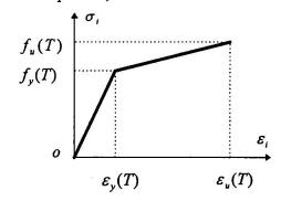
Figure 2  $\sigma_i - \varepsilon_i$  relations of the steel
