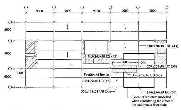
Fig. 1 General layout of test frame and position of first fire test.
