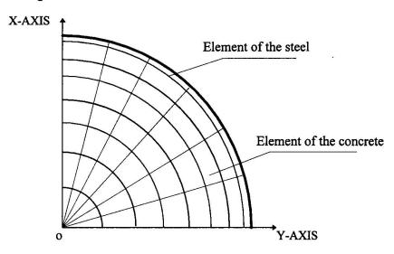
Figure 1 Arrangement of elements in quarter section
