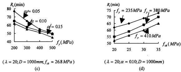
Figure 5 Influences of the parameters on the fire resistance time
