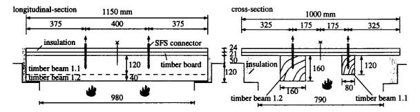
Fig. 9 Test arrangement for the tensile test of SFS-connectors subjected to the ISO-fire
