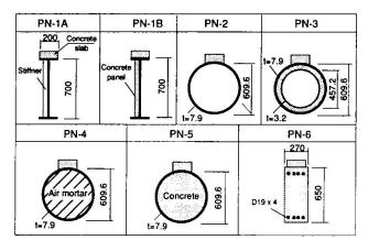
Fig.11 Test specimen
