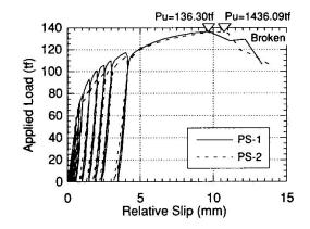
Fig. 10 Load and relative slip curve
