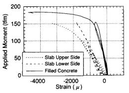
Fig.6 Concrete strain curves (T2)
