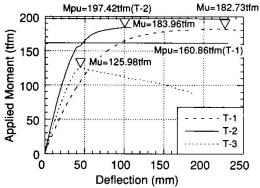
Fig.4 Moment displacement curve (T1 to T3)
