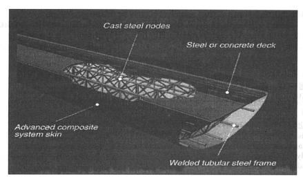
Figure 1 SPACES System Technology
