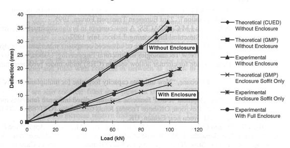
Figure 5 Comparison of experimental and theoretical results with and without participation of FRP shell
