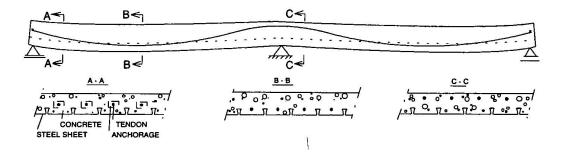
Fig.1. A composite slab with parabolic unbonded tendons.
