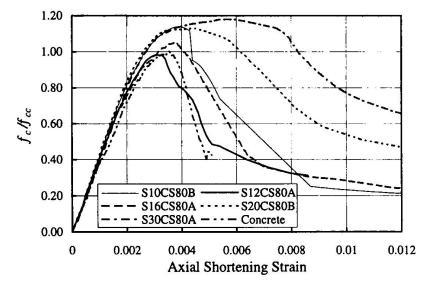
Figure 5 Confined concrete response for nominal 80 MPa mix
