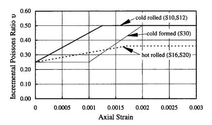
Figure 3 Poisson's ratio used in the analysis
