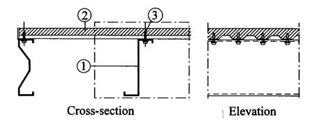
Fig. 1 Principle of the decking (showing structural components only): (1) purlins with a minimum thickness of 1.5 mm spaced at 600 mm, (2) concrete deck with a minimum thickness of 35 mm above the ribs (total depth 50 mm) and (3) screws as shear connectors.
