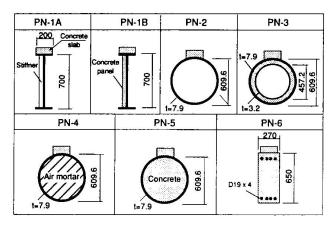
Fig.11 Test specimen
