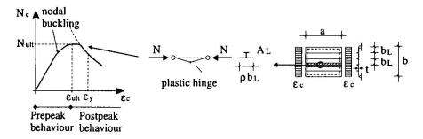
Fig. 4 Stiffened compression plates - strain oriented approach.
