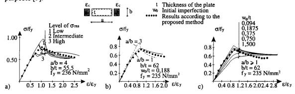
Fig. 3 Strain oriented effective width approach - comparison with test results: influence of a) residual stresses,  $\sigma_{res}$ , b) aspect ratio,  $\alpha/b$ , c) initial imperfections,  $w_0$ .
