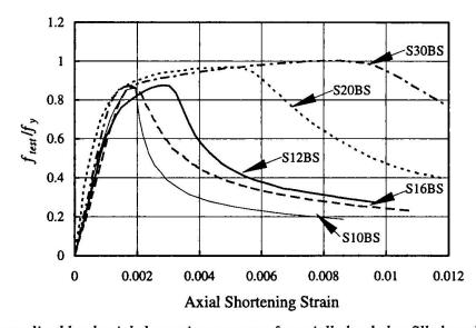
Figure 1 Normalised load axial shortening response for axially loaded unfilled steel tubes
