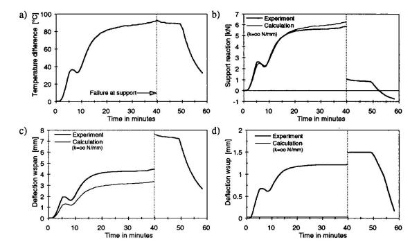
Fig. 2. Experimental and calculated  $(k = \infty)$  results of two-span test panel loaded by temperature difference in positive support reaction test. a) Temperature difference between the exterior and interior face, b) central support reaction, c) mid-span deflection and d) vertical displacement between the panel and the support structure at the central support. Dotted line shows the time point of local failure in the compressed external face at the central support.
