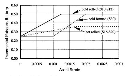
Figure 3 Poisson's ratio used in the analysis
