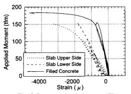
Fig.6 Concrete strain curves (T2)
