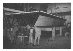
Figure 4 Cambridge half scale model of SPACES deck
