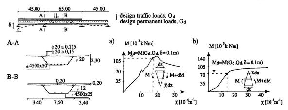
Fig. 1 Composite box girder bridge with typical cross-sections and their behaviour in terms of moment vs. curvature, a) at the support (section A-A), b) in the span (section B-B).
