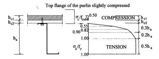
Fig. 5 Stress diagram at the termination of loading, as defined from the strain measurements.
