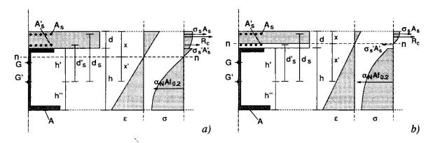
Fig. 3 Distribution of internal actions in the cross-section [a] x > d, b) x < d
