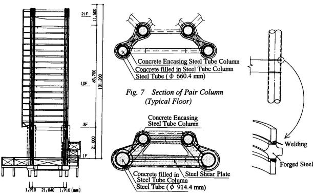
Fig. 6 Framing Elevation
