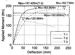
Fig.4 Moment displacement curve (T1 to T3)
