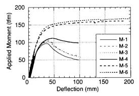
Fig.5 Moment displacement curve (M1 to M6)
