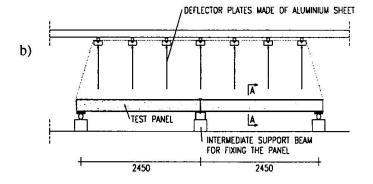
Fig.1. Loading arrangements in temperature loading tests.
