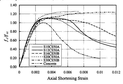
Figure 4 Confined concrete response for nominal 50 MPa mix
