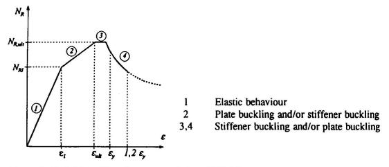
Figure 2. Model for stiffened compressed plate. RPX-95.
