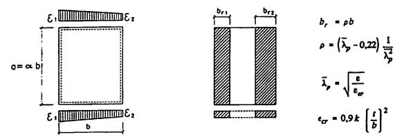
Figure 1. Model for slender compressed plates.
