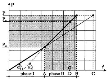
Fig. 5 Relation P = P(f) for phase I and II of a girder's work path. Notations: A, B, C, D - displacements of a middle point of a girder from: characteristic assembling load  $P_m$ , characteristic total load P - for a composite model, characteristic total load P - without accounting for concrete co-operation, characteristic real load  $P_a$
