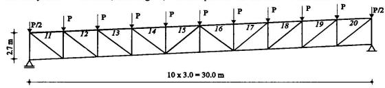
Fig. 4 Calculation scheme of truss girder
