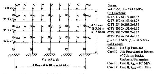
Figure 3: Composite CFT Frame Model
