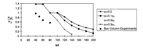
Fig. 5 Effect of Residual Stresses on Local Buckling Stress ( $\sigma_v$ =300 MPa; Pure Compression)
