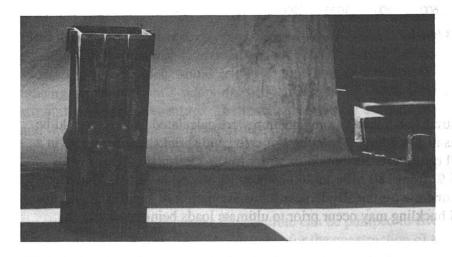
Fig. 4. Local Buckling Specimen NS5
