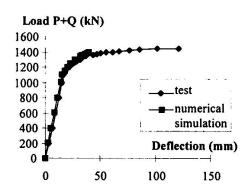
Fig.6 Comparison of the load-deflection curves
