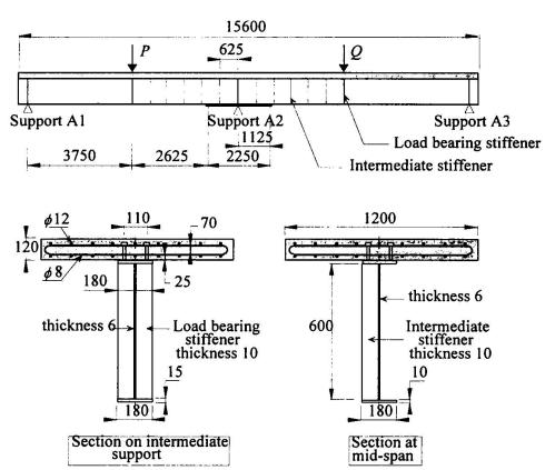
Fig. 1- Tested continuous composite beam
