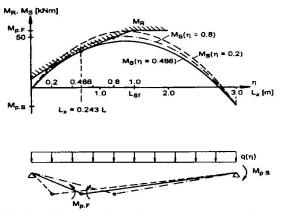
Fig. 2c:Design of continuous composite slabs
