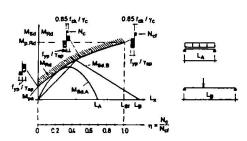
Fig. 2b:Design with partial interaction diagram
