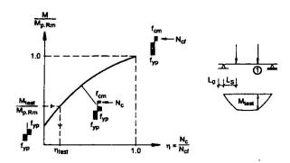
Figure 2a:Determination of the degree of shear connection from slab test
