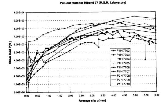
Fig 3 Shear-slip (P-u) curves for Hibond 77 from the pull-out tests (M.S.M. Laboratory)
