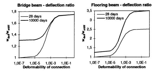
Fig. 4 Deflection ratio of the beams with deformable and stiff connection
