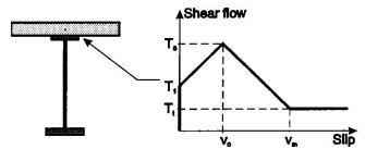
Fig. 2 The cross-section of composite beams studied and the idealized shear - slip diagram
