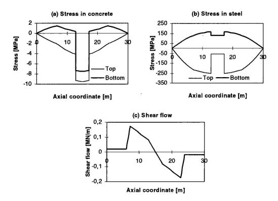
Fig. 3 Stress distributions and shear flow variation along the length of the beam
