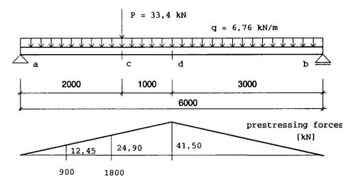
Fig. 2 Longitudinal section and values of prestressed forces
