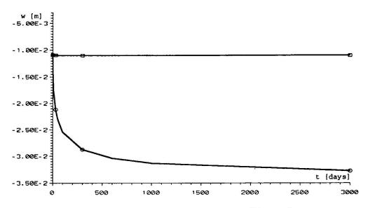
Fig. 4 Vertical deflections w(d,t) for case B,  $\square$  s/nc, O c/c
