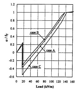
Fig. 5 Midspan section: progress of maximum stress in concrete and steel.
