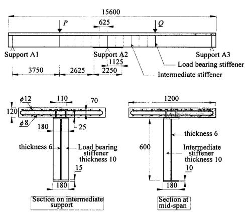
Fig. 1- Tested continuous composite beam
