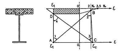
Figure 3. Ultimate strain conditions for Ultimate Limite State due to normal forces.
