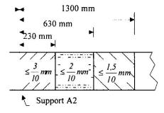
Fig. 4 Distribution of crack widths
