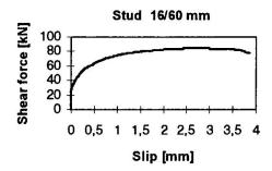
Fig. 1 Shear - slip diagram of one stud tested
