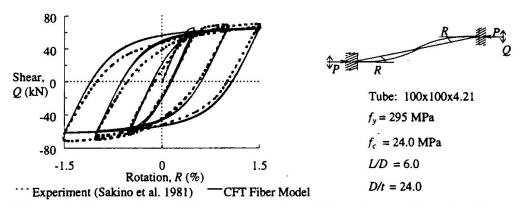
Figure 1: Comparison of Computational and Experimental Results (Sakino and Tomii 1981, Specimen CIVS3-2)
