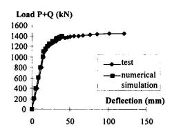
Fig.6 Comparison of the load-deflection curves
