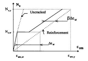
Fig.5 Tension stiffening curve
