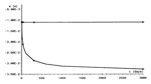
Fig. 4 Vertical deflections w(d,t) for case B,  $\square$  s/nc, O c/c
