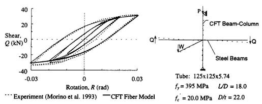
Figure 2: Comparison of Computational and Experimental Results (Morino et al. 1993, Specimen SCC-20)
