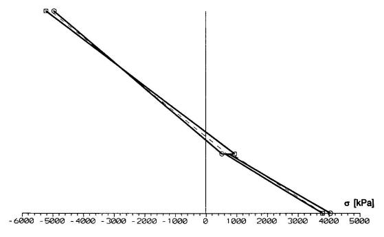
Fig. 5 Normal stresses  $\sigma_x(c,t)$  for case A;  $\square$  s/nc, O c/c. The full lines represent values  $\sigma_x(c,t\to\infty)$  and dashed line  $\sigma_x(c,t\equiv0)$
