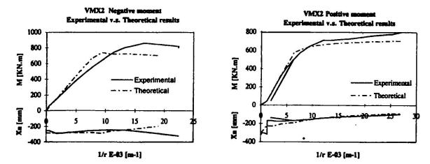
7.1 Support cross section 7.2 Center span cross section Figure 7. Moment-curvature diagrams. Experimental v.s. theoretical results.
