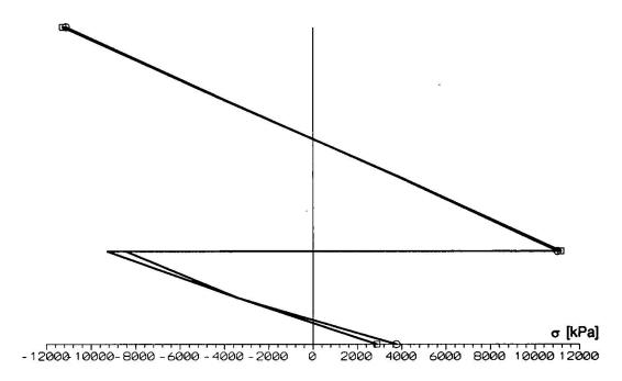
Fig. 6 Normal stresses  $\sigma_x(c,t)$  for case B;  $\square$  s/nc, O c/c. The full lines represent values  $\sigma_x(c,t\to\infty)$  and dashed line  $\sigma_x(c,t\equiv0)$
