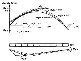
Fig. 2c:Design of continuous composite slabs
