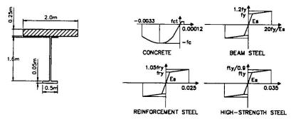
Fig. 1 Composite cross section and constituive laws.
