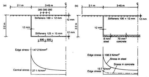
Fig. 5 Stress in an typical bridge girder. (a) Stiffened bottom flange, (b) Composite bot. flange
