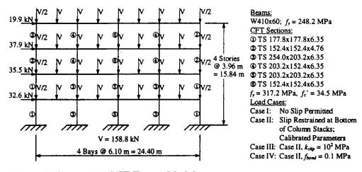
Figure 3: Composite CFT Frame Model
