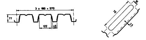
Fig. 2 Cross section and embossment pattern of Hibond 77 (all dimensions in mm)
