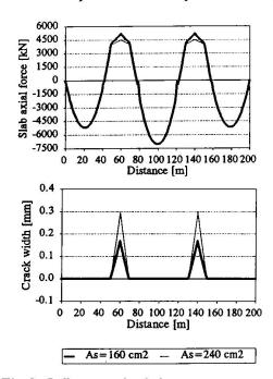
Fig.9 Influence of reinforcement on the slab behaviour
