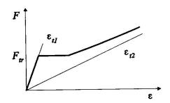
Fig.8 Constitutive relationship for concrete slab under tension
