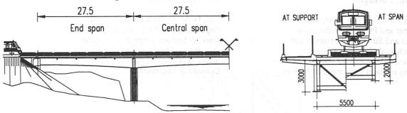
Fig.1 Longitudinal and cross section of a composite railway bridge over river Ave, Portugal
