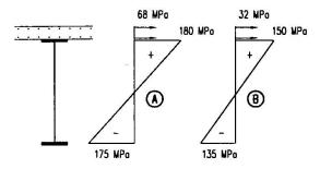
Fig. 7 Effects of the prestressing scheme
