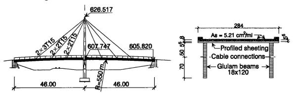
Fig.1: Cable-stayed footbridge, general layout and cross-section of the deck
