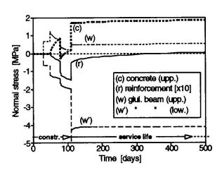
Fig.5: Normal stresses in the mid-section
