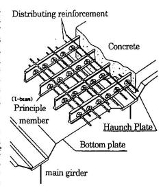
Fig.1 Structure of concrete-filled I-beam grid deck
