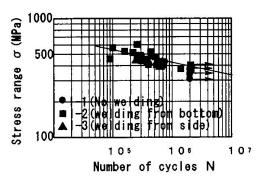
Fig.6 S-N curve for I-beam (crack initiation point)
