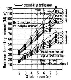
Fig.2 Relationships between slab span and maximum bending moment
