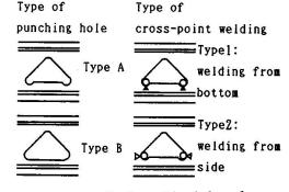
Fig.5 Details of punching hole and crosspoint-welding
