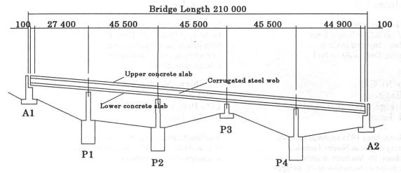
Figure-1 Side elevation of bridge
