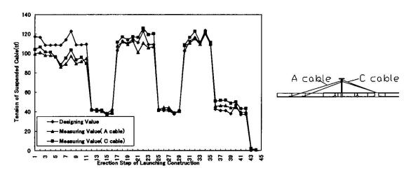
Figure-4 Tention change of diagonal suspension cables
