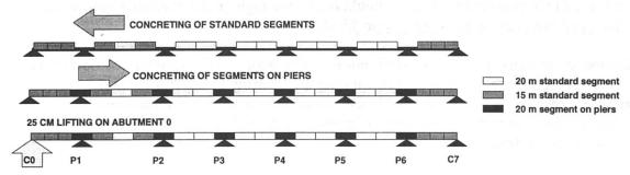
Fig. 3 Construction procedure by pilgrim's steps concreting
