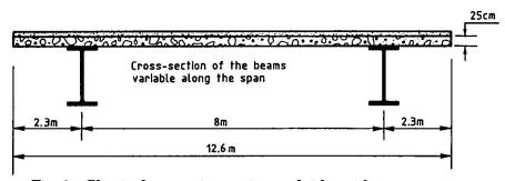
Fig. 2: Classical composite continuous bridge with two spans
