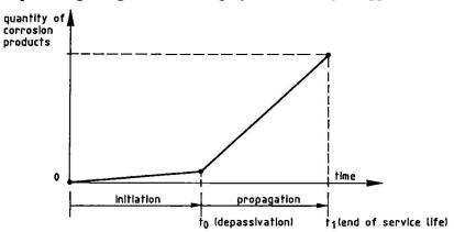
Fig. 1: Schematic representation of corrosion process
