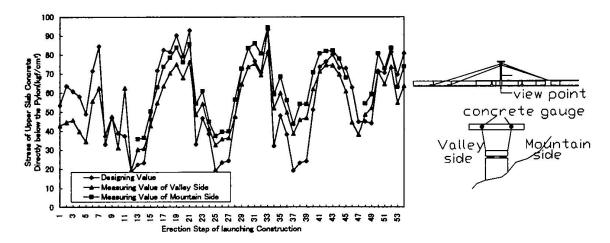
Figure-5 Stress change of upper slab concrete directly below the pylon
