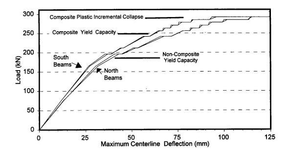
Figure 2 - Load vs. centerline deflection (West Span).
