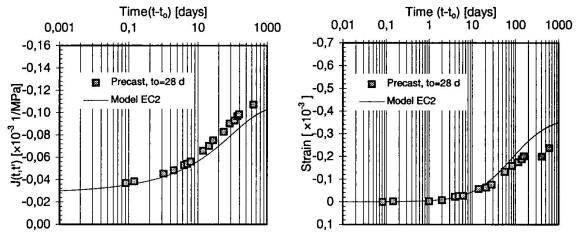
Fig. 3: Measured and calc.compliance function Fig. 4: Measured and calc. shrinkage strain of of precast concrete (type HC,  $t_0 = 28 d$ ) of precast concrete (type HC,  $t_0 = 28 d$ )
