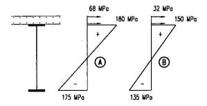
Fig. 7 Effects of the prestressing scheme
