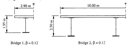
Figure 2: Typical bridge cross sections
