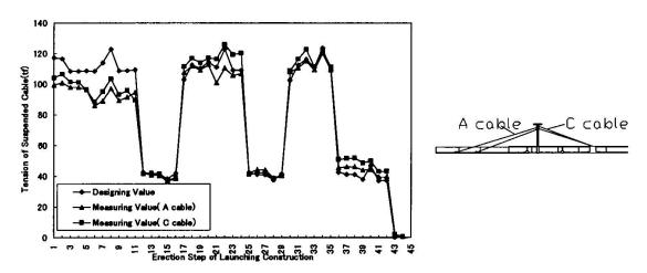
Figure-4 Tention change of diagonal suspension cables
