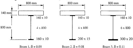
Figure 6: Geometry of tested beams
