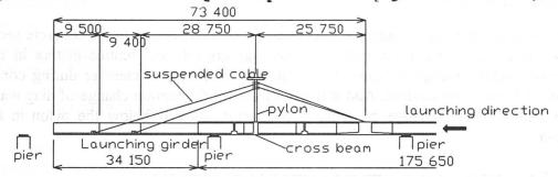
Figure-3 Set up of launching girder, Pyton and diagonally suspended cables
