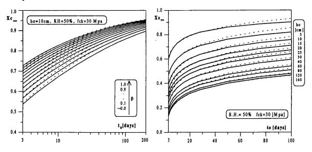
Fig. 1: a)  $\chi_{\infty}$  values for the imposed load problem. b)  $\chi_{\infty}$  values for the shrinkage problem.
