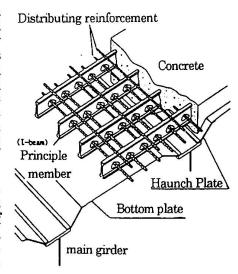
Fig.1 Structure of concrete-filled I-beam grid deck
