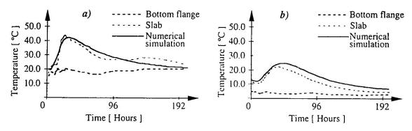
Figure 3: Temperature evolution: a) Bridge 1, b) Bridge 2
