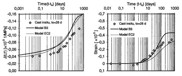
Fig. 5: Measured and calc.compliance function Fig. 6: Measured and calc. shrinkage strain of of cast in situ concrete (NC,  $t_0$ =28 d) of cast in situ concrete (NC,  $t_0$ =28 d)
