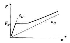
Fig.8 Constitutive relationship for concrete slab under tension
