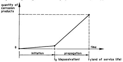
Fig. 1: Schematic representation of corrosion process
