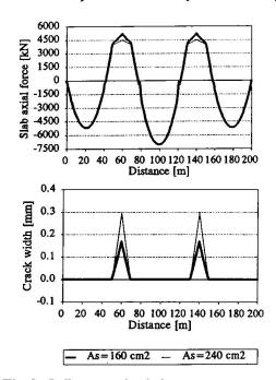
Fig.9 Influence of reinforcement on the slab behaviour
