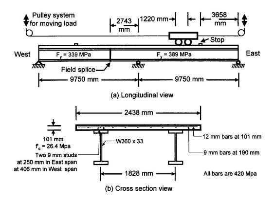
Figure 1 - Details of the test specimen.
