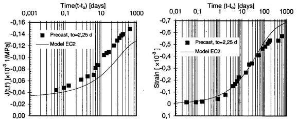
Fig. 1: Measured and calc.compliance function Fig. 2: Measured and calc. shrinkage strain of of precast concrete (type HC,  $t_0 = 2\frac{1}{4}d$ ) of precast concrete (type HC,  $t_0 = 2\frac{1}{4}d$ )
