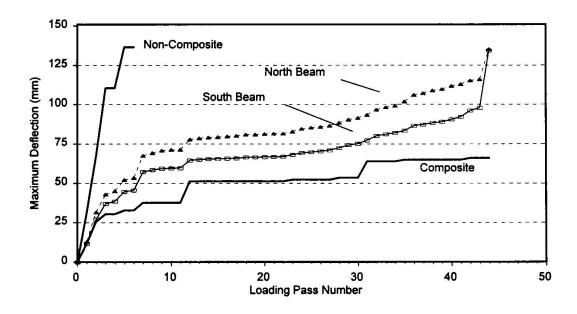
Figure 4 - Deflection vs. cycle number (East span).
