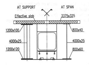
Fig.3 Viaduct cross section
