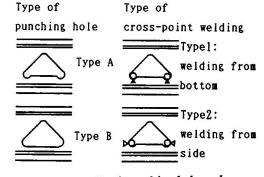
Fig.5 Details of punching hole and crosspoint-welding
