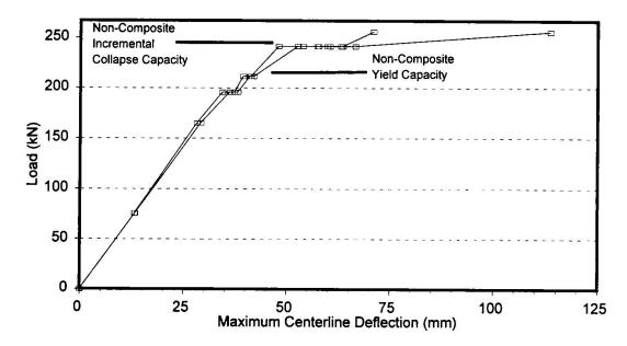
Figure 3 - Load vs. centerline deflection (East span).
