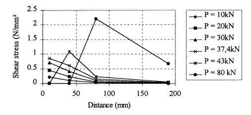
Fig. 2 Shear stresses of specimen A6 (100mm x 200mm)
