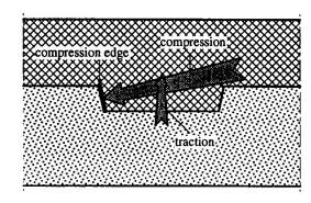
Fig. 5 - Detail: groove and post-tensioned HILTI-dowels
