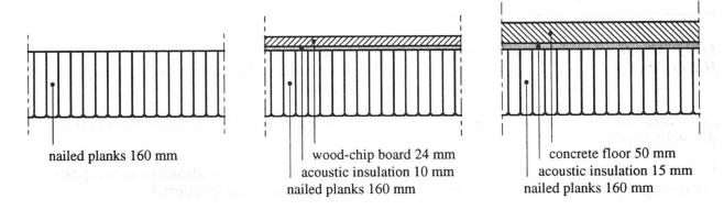
Fig. 4 - Examples of vertical nailed planks floor with different cover layers depending on specific requirements.
