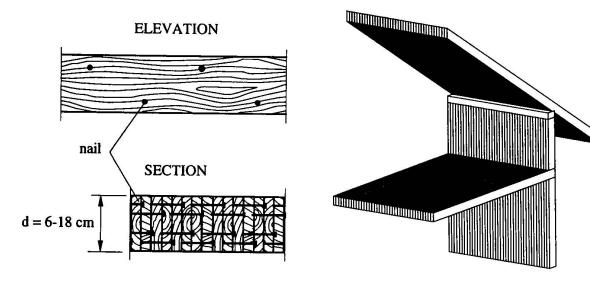
Fig. 1 - Nailing pattern for element construction.
