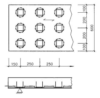
Fig. 4 Timber-concrete connection with grooved indentations in LVL
