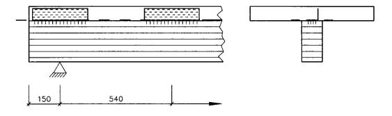
Fig. 2 Timber-concrete connection with punched metal plate fasteners
