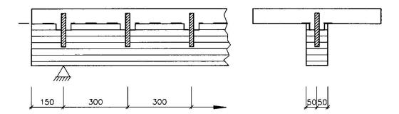
Fig. 3 Timber-concrete connection with grooved holes and dowels
