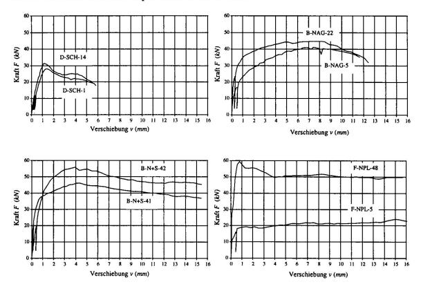
Fig. 5 Load-deformation-diagrams with maximum and minimum stiffness of four different connections. Screws (top left), punched metal plate fasteners (top right), grooved connections with dowels (bottom left), and grooved connections in LVL (bottom right)
