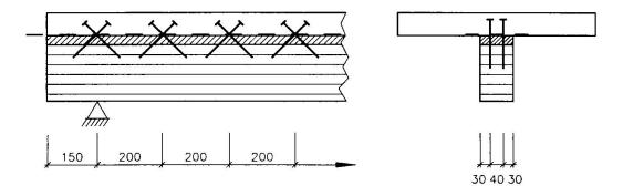
Fig. 1 Timber-concrete connection with crossed screws.
