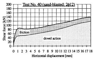
Fig. 5: Sand-blasted surface
