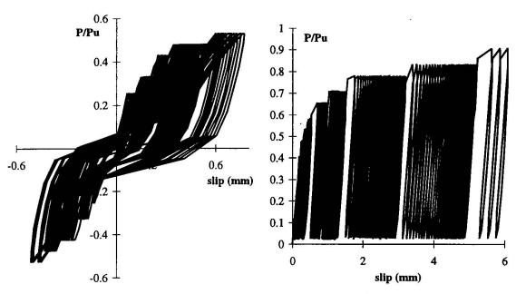
Fig. 2 Load versus slip plots for symmetric cyclic (test 15 - left) and unidirectional cyclic (test 13 - right) loading
