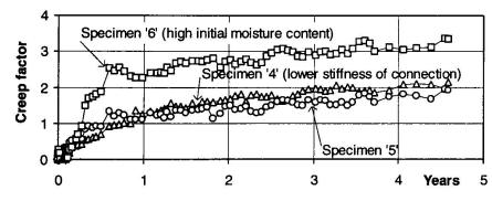
Fig. 2. Creep of three different TCC-specimens
