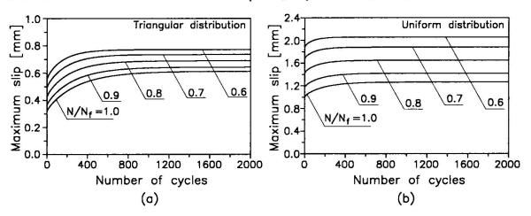
Fig. 4 - Maximum slip versus number of cycles: triangular a) and equally spaced studs b).
