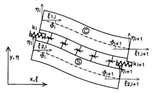
Fig. 1 - Four noded finite element.
