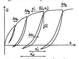
Fig. 2 - Load-slip curves (Q-s) of a connector for repeated loading.
