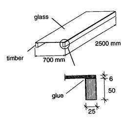
fig.I: composite element timber-glass
