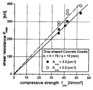
drop shaped concrete dowels
