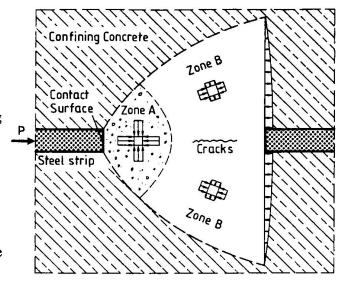
Fig. 6 Loading of a Concrete Dowel
