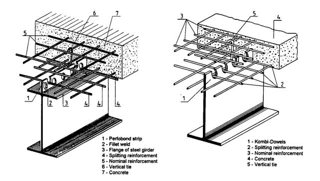
Fig. 1 Composite beam with Perfobond Strip
