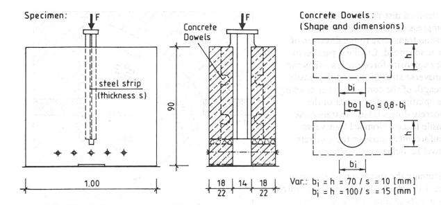
Fig. 3 Push-out test specimen and investigated variants of Concrete Dowels
