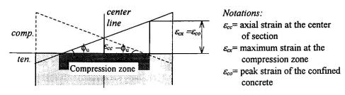
Fig. 1 Idealization of the strain distribution of column section under cyclic moment
