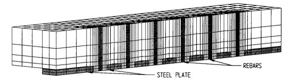
Fig. 4. Three-dimensional finite element model.
