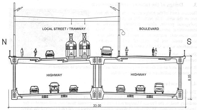
Fig. 1 Cross-section of bridge with the traffic areas
