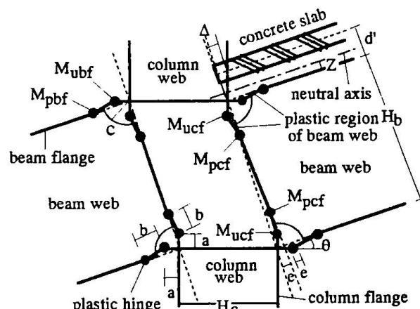
Fig.2 Plastic deformation of the connection
