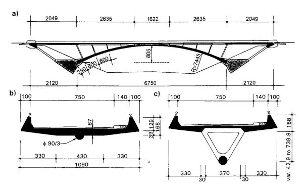
Fig. 1 Structural solution: a) elevation, b) cross section at midspan, c) typical section
