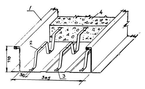
Fig. 1. Anchor connectors in composite slabs
