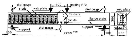
Fig. 1 Setup for test and a specimen (Model A-1)
