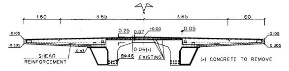
TRANSVERSE CROSS SECTION (REINFORCEMENT IN SITU CONCRETE)
