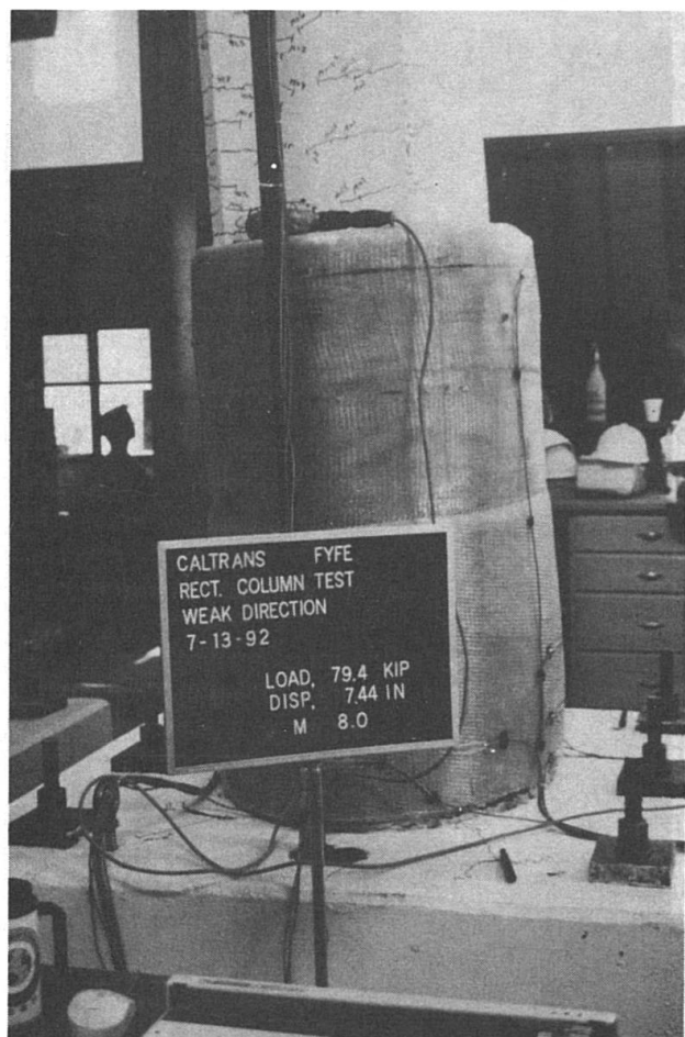
Figure 3 Epoxy-Fiberglass Column Wrap in Laboratory Test Figure 4 Field Application
