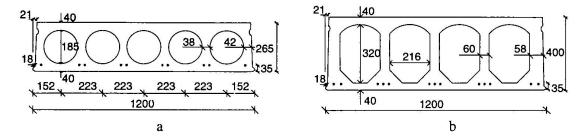
Fig. 3 Nominal cross-section of slabs. a) Tests DE265, ST265, PC265E, PC265E, PC265T, PC265N, PC265C, RC265. b) Tests PC400, ST400
