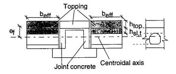
Fig. 5 Composite beam model
