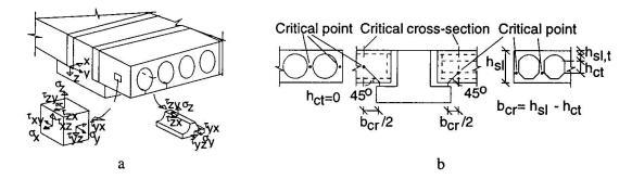
Fig. 4 Stress components in the web
