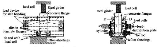
Fig 7: Test set-up and test specimen for push- Fig. 8: Sectional view of test set-up and out tests specimen for push-out tests.
