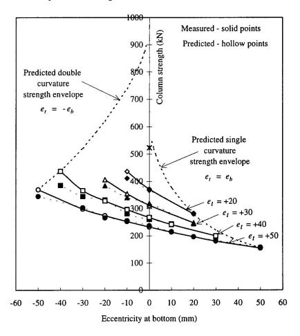
Figure 1 Measured and predicted column strengths
