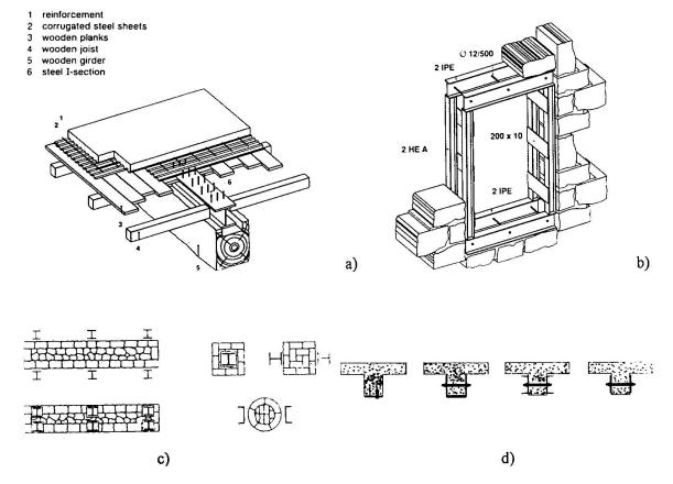
Fig. 10. Technologial systems based on composite actions, which are commonly used in consolidation operations: a) composite steel-timber floor; b) steel frame in a masonry opening; c) steel reinforcement for masonry walls and columns; d) integration of RC sections with steel plates.
