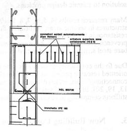
Fig. 4. Composite MRF subsystem made of RC columns and steel-RC composite beams.
