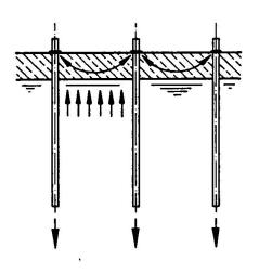
Fig. 2: Simple computational model for the verification of underwater slabs
