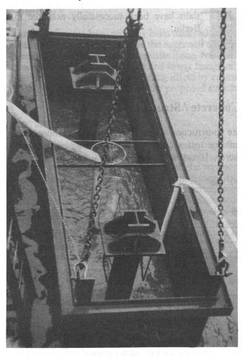
Fig. 6: Steel container with two pile heads
