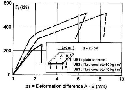
Fig. 3: Results of test loading - plates with plain and steel fibre concrete
