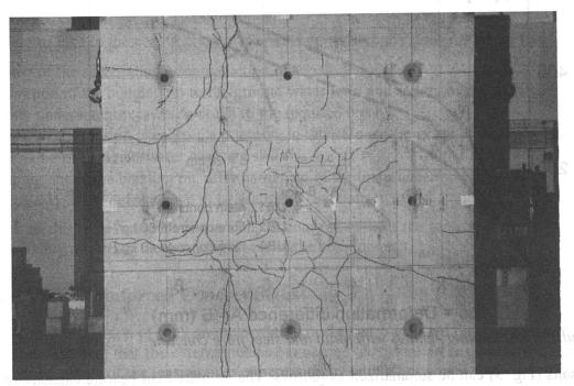
Fig. 5: Specimen with steel fibre content of 40 kg/m<sup>3</sup> concrete and behaves a serious misle
