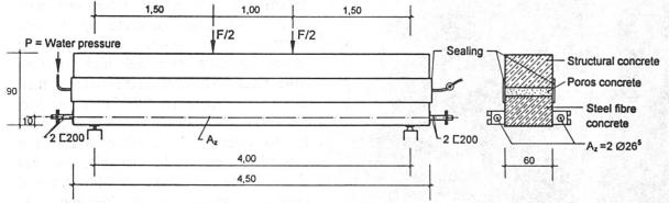
Fig. 8: Composite beam test set-up
