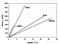
Fig. 2 Stress / strain diagram for FRP materials used
