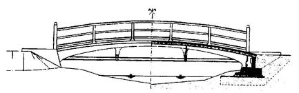
Fig. 3 Elevation and longitudinal section of the trial bridge
