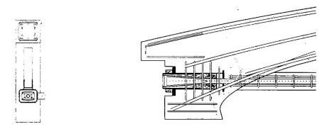
Fig. 5 Arrangement of strain gauges at midspan
