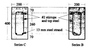
Fig. 1 Cross-section of beam specimens
