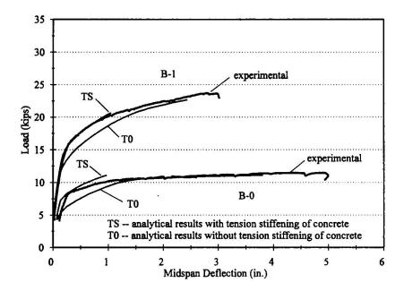
Fig. 3 Experimentally observed and predicted load-midspan deflection for B-0 and B-1
